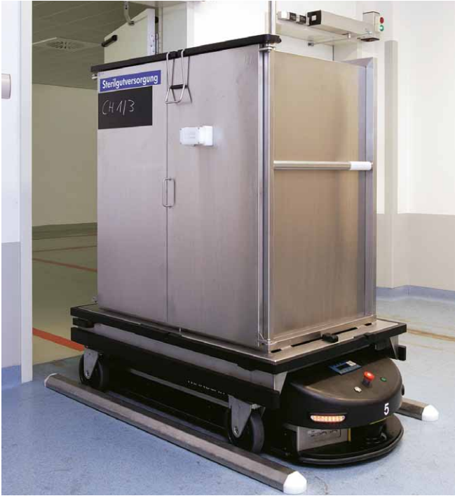
AGV transport cart is collected automatically
