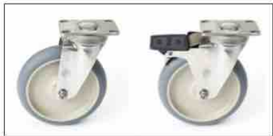
All stainless steel construction. Grease sealed stainless steel ball-bearings with zerk fittings. Available in 6" (152 mm) diameter, swivel, brake-lock and swivel-lock tracking options. Rounded wheel tread provides less surface contact, improving rollability. Softer tread absorbs more energy while rolling — reducing overall cart noise.
